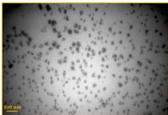
Fig. 2. TEM image of synthesized CURNs.
